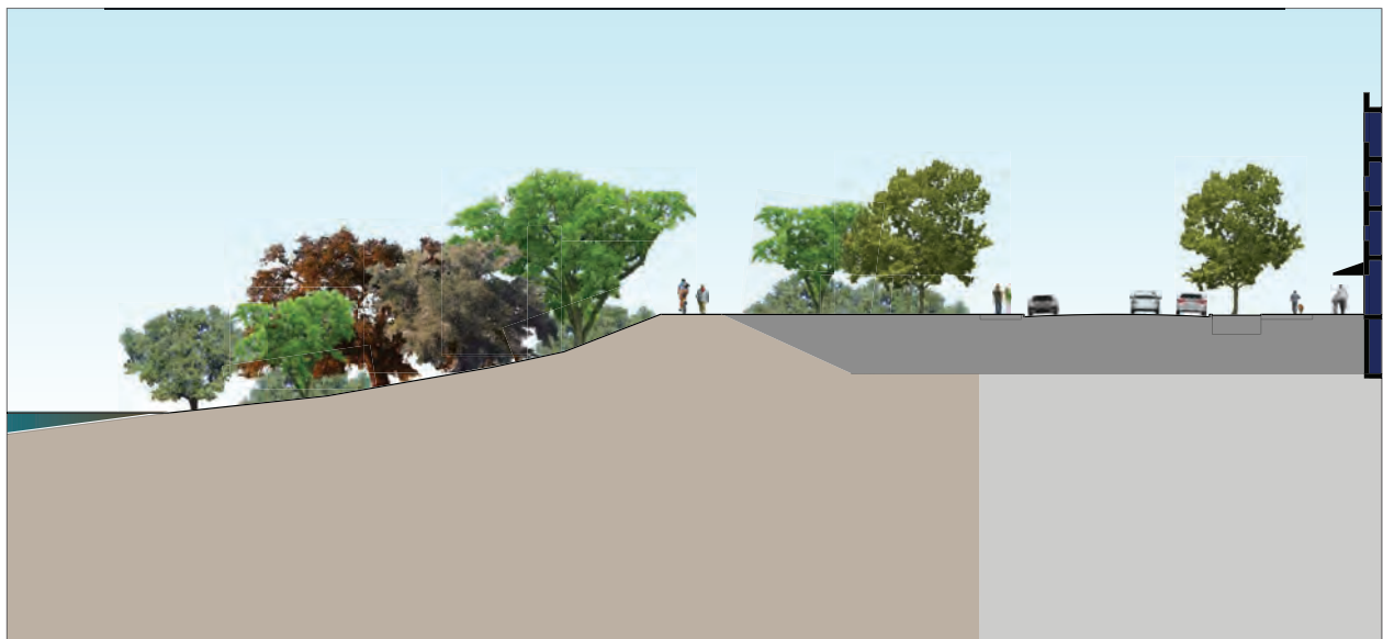
FIGURE 6.10 Township 9 will berm up to the levee top.
